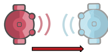
Fig. 2. One-way coupling: "Live" agent (red) tested or evolved with a "ghost" agent (blue). Live agent is sending and receiving acoustic signals. Ghost agent is playing back pre-recorded behavior of previous trials and so sending pre-recorded signals but not receiving anything.
